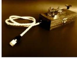
The Tworse Key is a standalone device that connects through a standard LAN cable, the Morse signals are decoded by the built-in Arduino Ethernet board, which delivers the final message through the Twitter API. Please follow [@tworsekey](#) on Twitter to read some example tweets sent from the actual device
